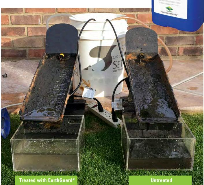
**Temporary Erosion Control EarthGuard® Soil Stabilizer**
